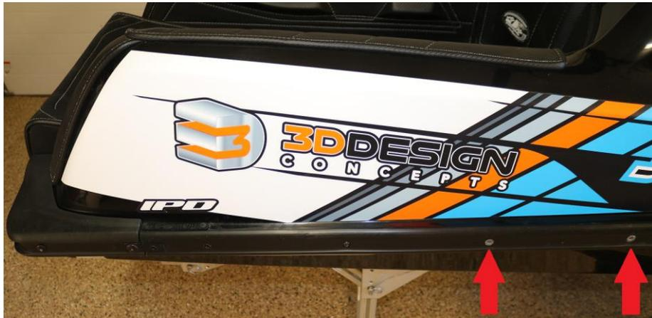
3. Attach the connected mid sponsons (or the filler plates if you didn't order the connected mid sponsons) to the base sponsons using 2X M5 flat head screws on each side.
